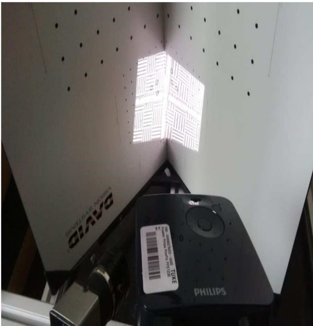
Figure 1 The projector and camera calibration with laser scanner DAVID
