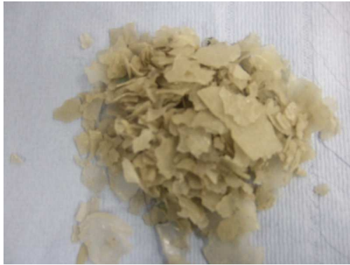
Figure 2 Recycled polyvinyl butyral [7]
