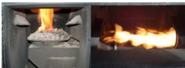
Figure 1 Flame direction – retort burner on the left, tube rotary burner on the right
