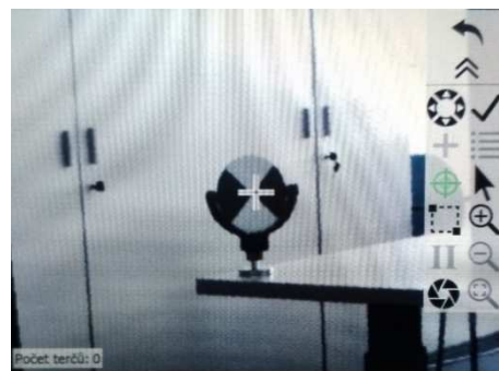
Figure 5 Targeting of reference target
