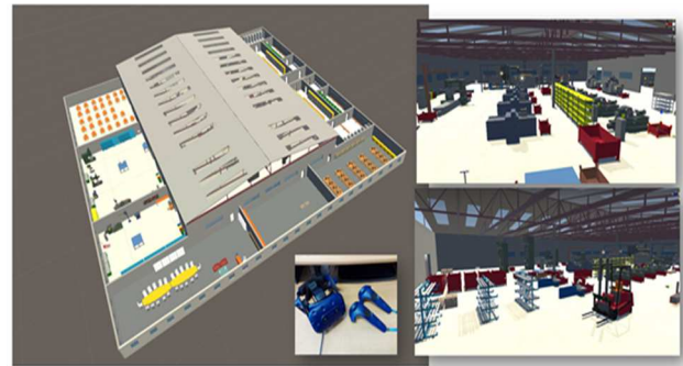
Figure 2 Design of production system in virtual reality using HTC Vive Pro and Unity 3D
