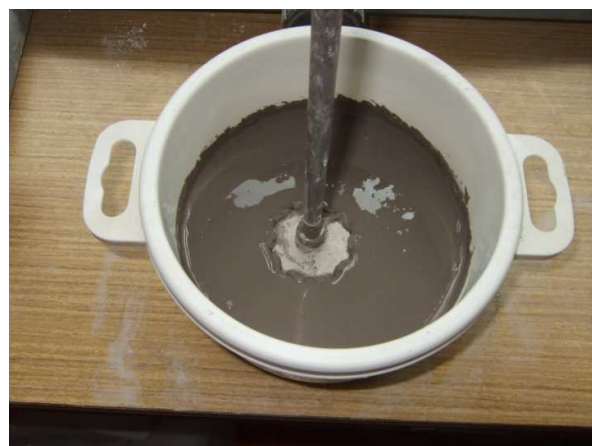
Figure 2 Homogenization of geopolymer composite material [authors own processing]
