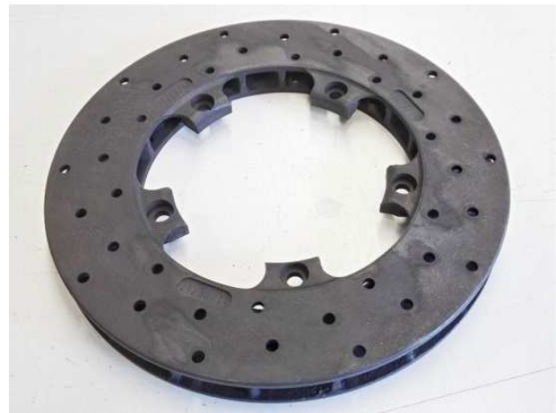
Figure 2 Brake disc with surface treatment phosphate of zinc
