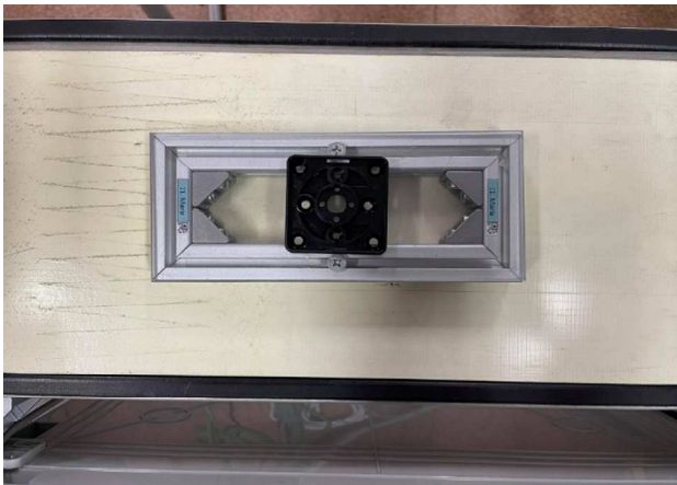
Figure 4 Pallet with measured workpiece on automated line
