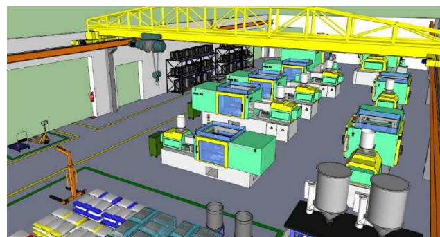
Figure 5 View of the proposed bridge crane
