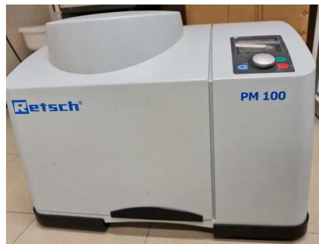
Figure 1 Planetary ball mill Retsch PM100 (in Institute of Physics, Faculty of Science, P. J. Šafárik University in Košice)
