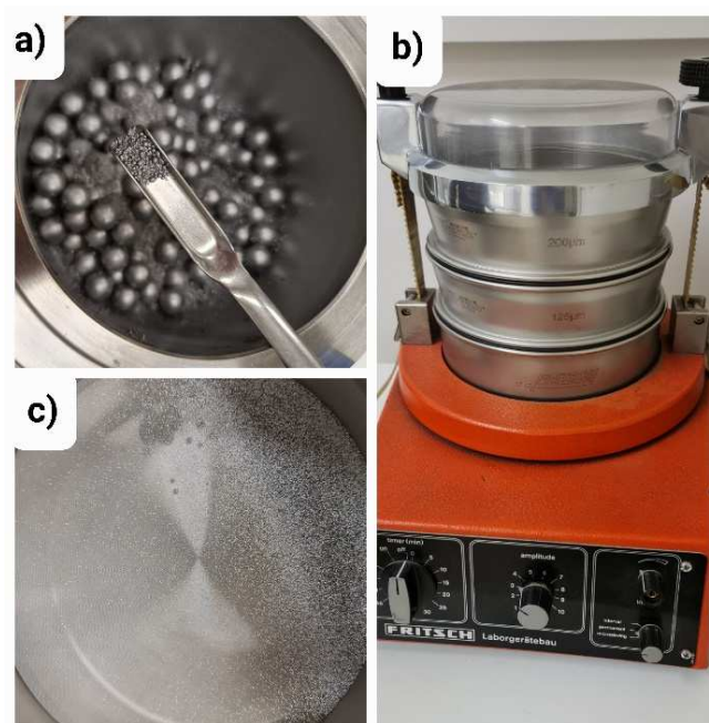
Figure 2 a) powder after mechanical milling at milling vessel, b) vibrating mill FRITSCH with sieves, c) powder after sieving (in Institute of Physics, Faculty of Science, P. J. Šafárik University in Košice)
