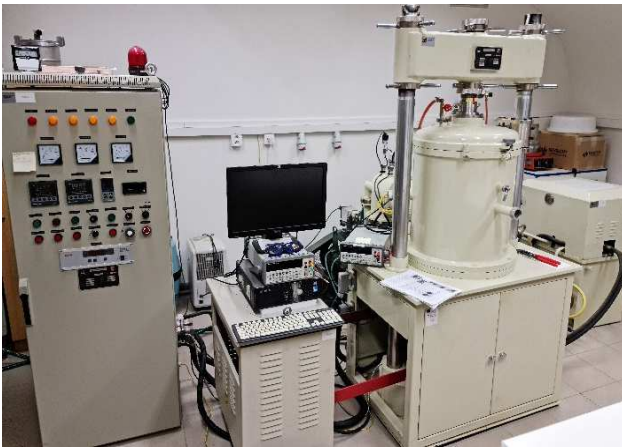
Figure 4 LTVAT ZT-25-20Y machine for the compaction (in Institute of Physics, Faculty of Science, P. J. Šafárik University in Košice)
