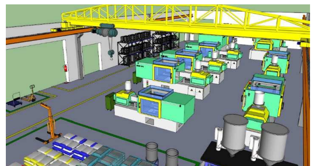
Figure 5 View of the proposed bridge crane
