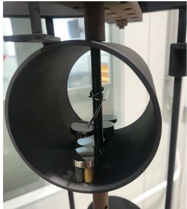
Figure 2 Placement of samples in a tube-shaped fixture ( L=100 mm) with the cathode in the axis of the tube in a vacuum chamber
