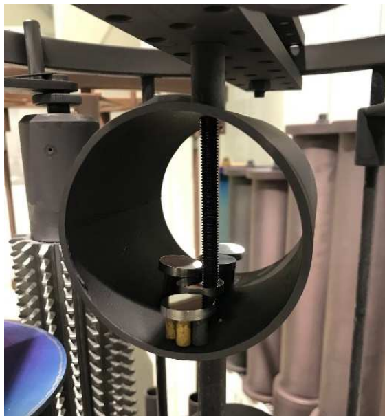
Figure 1 Placement of samples in a tube-shaped fixture ( L=100 ) without a cathode in the tube axis in a vacuum chamber
