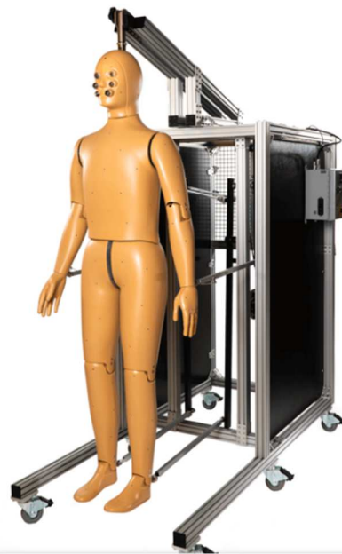
Figure 3 ANDI manikin for clothing testing [13]
