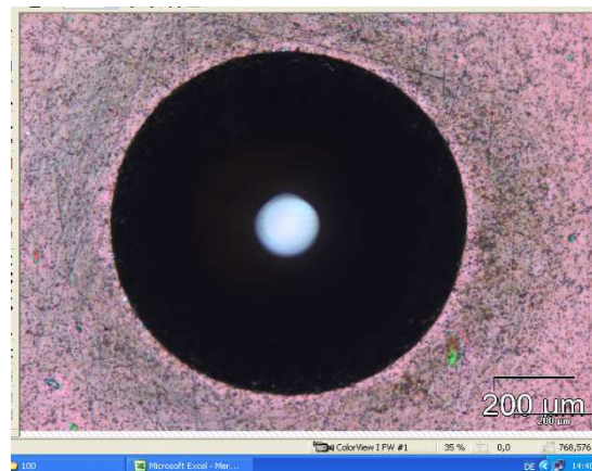
Figure 10 Puncture after Mercedes test HF level 2
