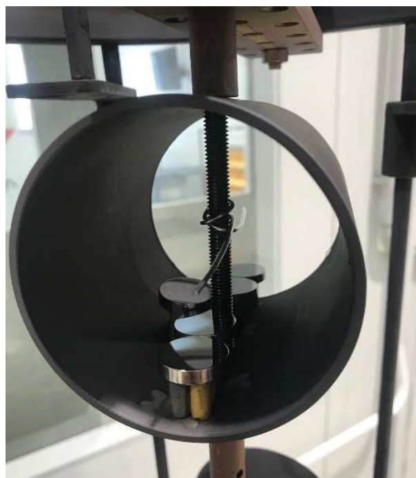
Figure 2 Placement of samples in a tube-shaped fixture ( L=100 mm) with the cathode in the axis of the tube in a vacuum chamber
