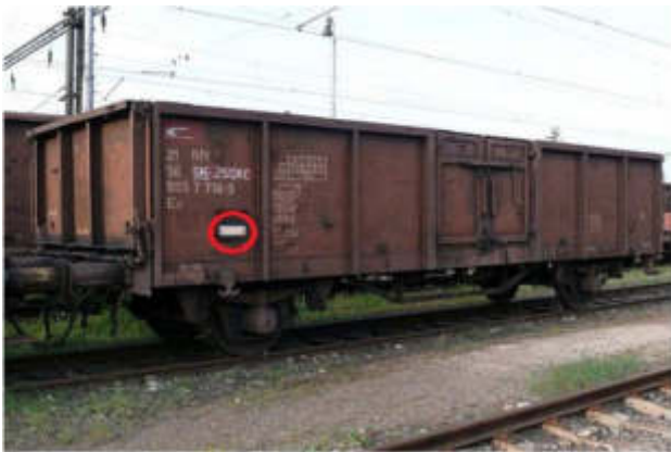
Figure 2 Application of RFID tag in real conditions of railway cargo transport
