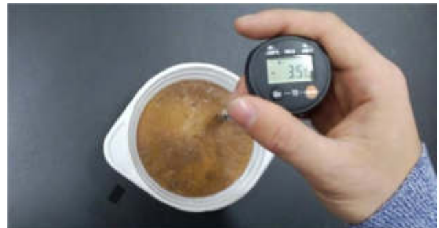
Figure 3 Displaying the the magnesite powder coating layer on the surface of the RFID transponder 20 mm thick with the addition of water in a ratio of 1: 1 (g / ml), followed by freezing at -3.5 ° C
