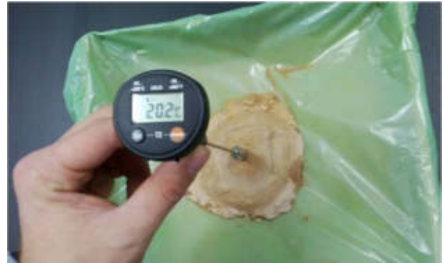
Figure 2 Displaying the the magnesite powder coating layer on the surface of the RFID transponder 20 mm thick with the addition of water in a 1: 1 (g / ml)
