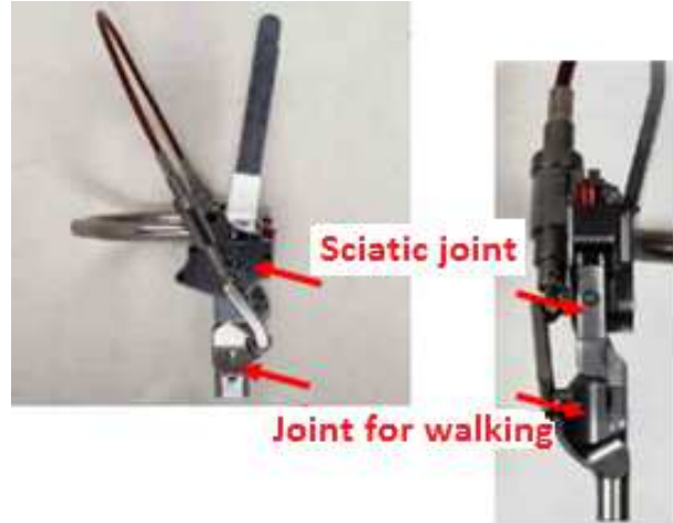
Figure 2 Sciatic joint and joint for walking
