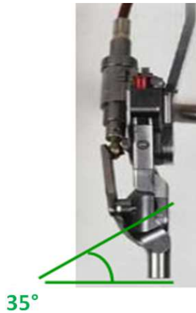
Figure 4 Axis joint with 35 ° inclination
