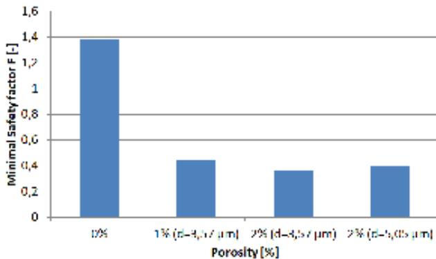
Figure 4 Minimal Safety factor  $F$  for 0% (free porous FE model), 1% and 2% porosity. 2% porosity with 20 pores  $d=3,57 \mu\text{m}$  gives the smallest safety factor. The highest safety factor is calculated for free porous FE model
