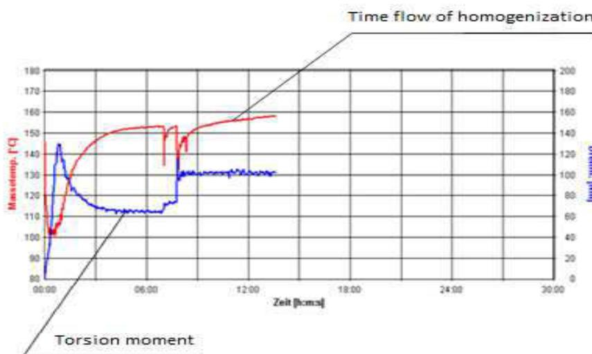
Figure 3 Polyvinyl butyral homogenization [9]
