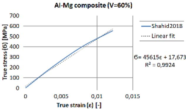
Figure 2 Al-Mg hot-pressed, reactive sintered composite with Mg volume content  $V=60\%$ . Measured data is taken from [3]. Measured data is linearly fitted with a resulting coefficient of determination  $R^2$  greater than 0.99
