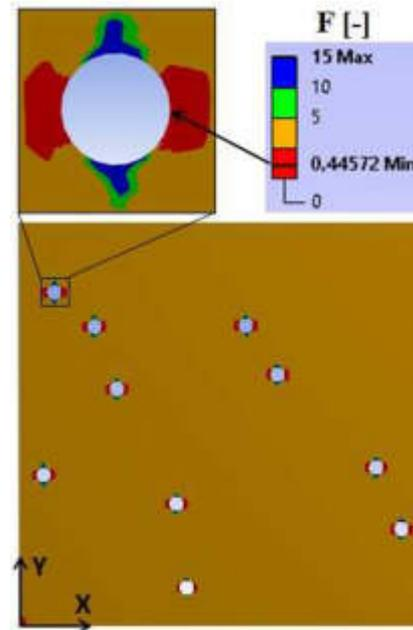
Figure 3 Safety factor  $F$  distributions in FE model with detailed view on the most critical position. Minimum calculated safety factor  $F=0.44572$  corresponds with maximum principal stresses approximately of 1288 MPa. Safety factor (stress) distribution is similar around all pores in the FE model
