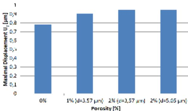
Figure 5 Maximal displacement  $U_y$  for 0% (free porous FE model), 1% and 2% porosity. 2% porosity with 10 pores  $d=5.05 \mu\text{m}$  gives highest displacement. Smallest displacement is calculated for free porous FE model
