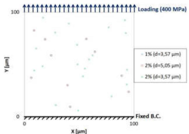
Figure 1 Scheme and size of the FE model. Legend describes the size of the pores in the FE model. 1% and 2% porosity is created in the FE model by varying the pore diameter  $d$  and number of pores. FE Model is loaded on the top edge with tensile load  $400 \text{ MPa}$
