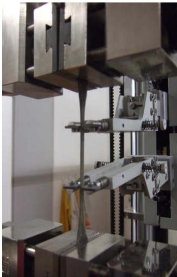
Figure 4 Tensile test of recycled polyvinyl butyral [9]
