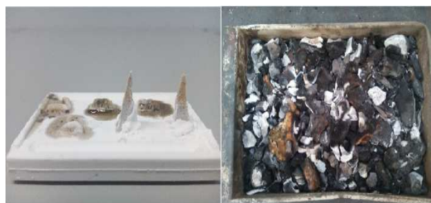
Figure 5 Ash melting point test and imperfectly burned bones
