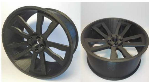
Figure 10 Physical model made by 3D printing
