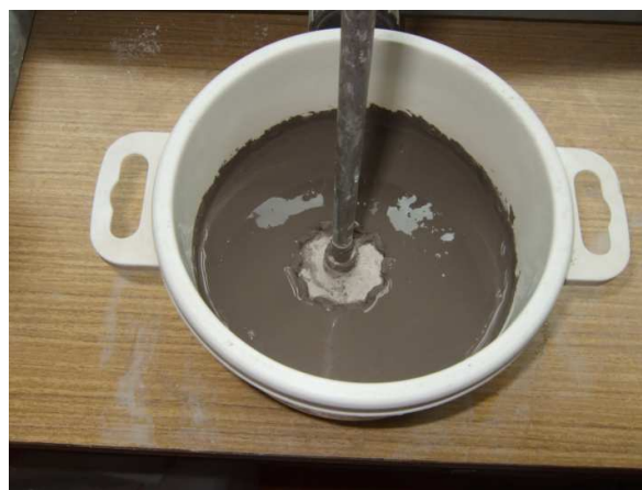
Figure 2 Homogenization of geopolymer composite material [authors own processing]
