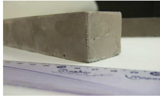
Figure 4 Geopolymer reinforced with fabrics from waste tyres [authors own processing]
