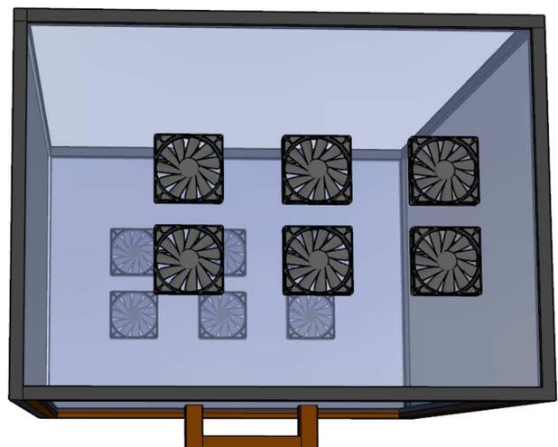
Figure 3a Laminar box design
