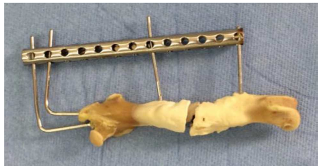
Figure 6 Explanted personalized fixation with overgrown implant structure
