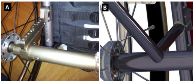
Figure 3 Center of gravity before (A) and after adjustment (B)
