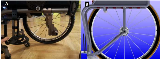
Figure 4 Frame before (A) and after modification (B)
