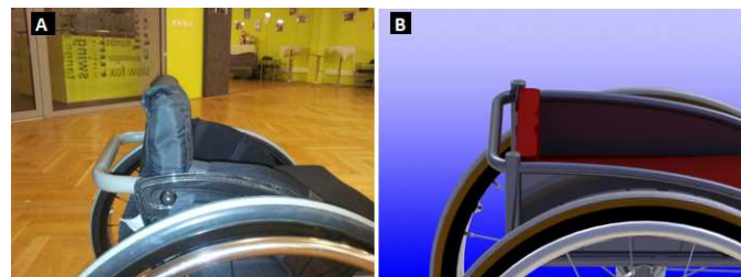
Figure 8 The original height (A) of the backrest and its reduction (B)
