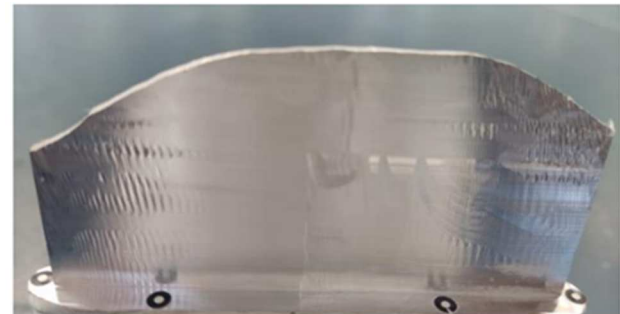
Figure 3 Thin-walled part after milling by end mill with helix angle 25°
