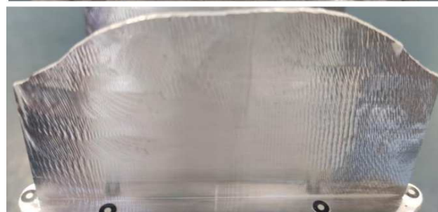
Figure 4 Thin-walled part after milling by end mill with helix angle 30°
