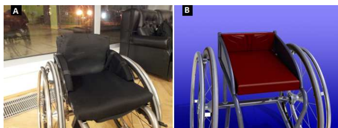
Figure 7 Original (A) and modified seat (B)
