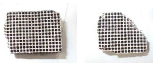
Figure 5 Pieces from catalyst number 3 [3]
