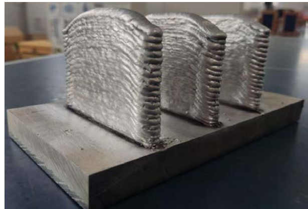
Figure 1 The sample manufactured by the WAAM technology
