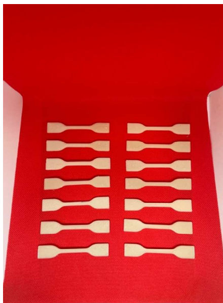
Figure 7 Final printed samples using FFF technology
