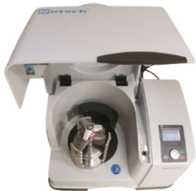
Figure 3 Planetary ball mill Retsch PM100 (in Institute of Physics, Faculty of Science, P. J. Šafárik University in Košice)
