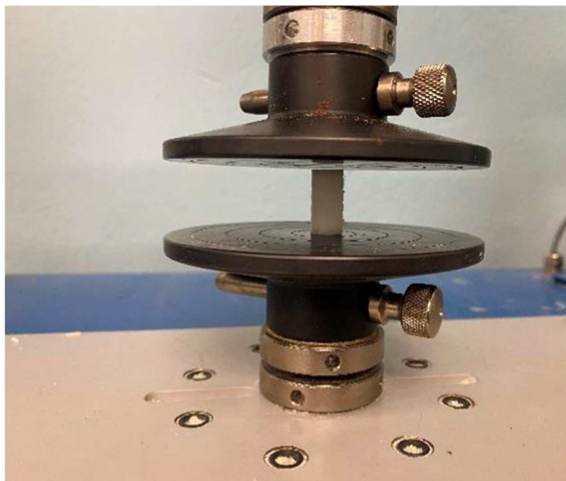
Figure 5 Test sample inserted between jaws
