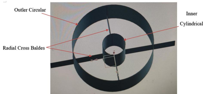
Figure 2 Cutting mechanism design
