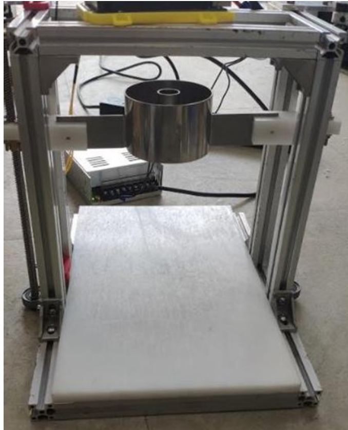
Figure 6 Assembled prototype of the pineapple cutting machine
